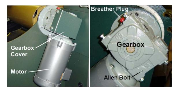
Use 265ml to 325ml (9 to 11 ounces) of oil per gearbox for your EC-1. Due to the mounting configuration, the window on the gearbox cannot be used to monitor the amount of oil however you must ensure that the gearbox is never more or less then half filled with oil at all times! Quaker State Synthetic Gear Oil is recommended but any brand between 75W to 90W Synthetic Gear Oil or Synthetic High Pressure Gear Oil is acceptable.
