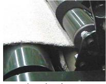
While gently holding this Handle in place, press the Jog Button to continue the advancement of the carpet. You will only have to hold the Handle in place for 1 or 2 seconds at which time you will see the plates actually force the carpet around the core. Once you see the carpet is starting to wrap around the core, release the Handle to its original position.
