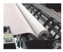
IMPORTANT NOTE: IF YOU CONTINUE THE ROLL-UP PROCEDURE BY PRESSING THE JOG BUTTON INSTEAD OF THE FOOT CABLE, THE MACHINE WILL NOT STOP AUTOMATICALLY AT YOUR PRE-SET LENGTH. BE SURE TO USE THE FOOT CABLE AFTER YOU HAVE STARTED THE CARPET SO THIS FUNCTION CAN PERFORM PROPERLY.
