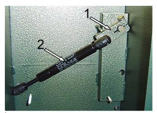
This photo of a Machine (with the Counter and Switches removed) shows the Counter Weight Bracket (#1) lined up with the Shock (#2) at a 45 degree angle. This is what the assembly should look like with the Counter Weight Wheel in the **UP** position.
