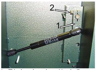
➤ This photo shows the position the Counter Weight Bracket (#1) should be in with the Counter Weight Wheel in the **DOWN** position. To make your adjustment loosen the Bolt (#2) and put your Counter Weight Wheel Down so the Bracket is in this vertical position.
