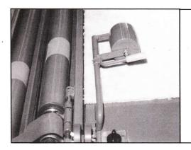
As carpet rolls towards the left hand rollers, guide carpet underneath the counter weight and stop at cutting bar edge. This will tell you if carpet edge is straight. If not adjust roll accordingly - manually.
