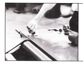
To cut the floor material engage cutting bar by turning control switch to forward position to engage cutting process. Once the flooring is cut return blade by turning switch to reverse.
