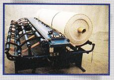
The advanced cradle system is equipped to handle both carpet and vinyl flooring.
