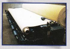
The use of a core provides a secure roll up while the operator watches and inspects the flooring.
