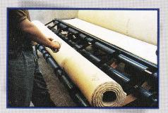
With operating cables around the entire machine, wrapping both the cut and balance rolls is done very easily.
