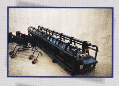
The machine arrives fully assembled with the exception of the support stands and caster wheels.
