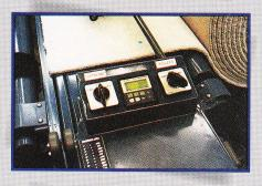
The electronic counter provides accurate inventory counts and gives you the ability to detect shortages.
