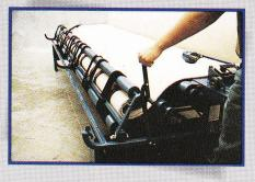
The spring-loaded receiving cradle allows for an easy and tight roll up of all flooring.
