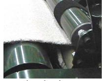
While gently holding this Handle in place, press the Jog Button to continue the advancement of the carpet. You will only have to hold the Handle in place for 1 or 2 seconds at which time you will see the plates actually force the carpet around the core. Once you see the carpet is starting to wrap around the core, release the Handle to its original position.
