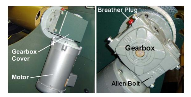
Use 9 to 11 ounces of oil per gearbox for your EC-1. Due to the mounting configuration, the window on the gearbox cannot be used to monitor the amount of oil however you must ensure that the gearbox is <u>never more or less then half filled with oil at all times!</u> Quaker State Synthetic Gear Oil is recommended but any brand between 75W to 90W Synthetic Gear Oil or Synthetic High Pressure Gear Oil is acceptable.
