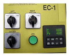
➤ Check that the Cutting Bar is working by pushing & holding the Cutter Switch to FWD. Since it is a Two-Way Cutter, you can make your next cut by pushing & holding the Cutter Switch to REV.
