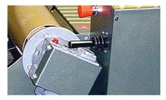
middle of the Load Side Cradle. This feature will actually "twist" the roll of carpet that is in the Load Side Cradle so as to shift if from the back of the machine towards the front, or vice-versa, depending on which direction you move the toggle switch. This process will aid the roll-up of your carpet in the event that you have a roll that tends to walk or telescope.
