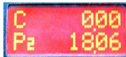
➤ For Example if you need to make an eighteen and a half foot cut, simply program the Pre-set Length in the P2 Screen to read “18.06”.
