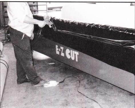
To roll, wrap or tape floor covering, disengage cutting blade by pushing the right clutch bar down to disengage position. This will allow the roller on the left hand side to roll freely. This can be controlled by the hand control switch or by the foot pedal switch.
