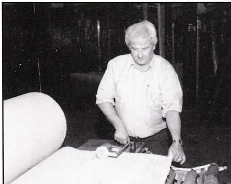
As you start rolling the flooring, guide the floor covering by pulling gently on the edge of the carpet with your left hand, as shown on photo
