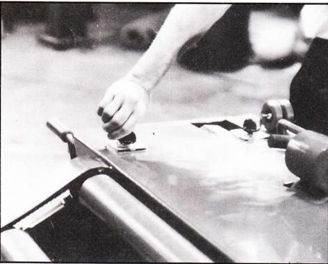
To cut the floor material engage cutting bar by turning control switch to forward position to engage cutting process. Once the flooring is cut return blade by turning switch to reverse.
