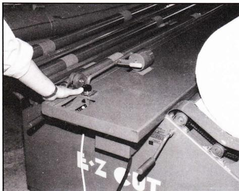
Place roll of carpet or vinyl flooring on the machine. Please ensure the feed is coming from the bottom towards the counter. Advance carpet forward or reverse by the hand control switch.
