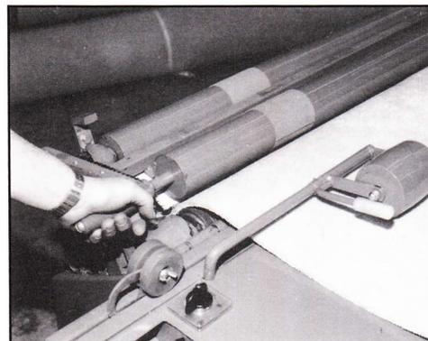
Close rollers as shown to ensure proper rolling start. (photo at left).
